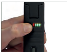
battery test button
