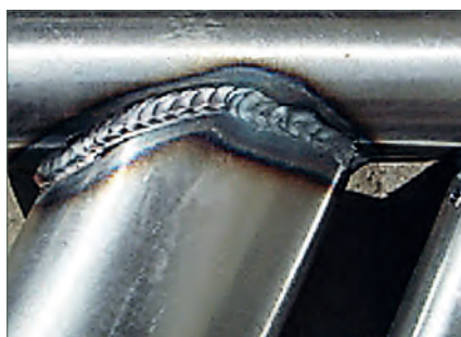
TIG, flat welding, carbon steel, 130amps
