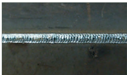
CO2 MIG, flat welding, carbon steel, 130amps
