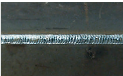
CO2 MIG, flat welding, carbon steel, 130amps
